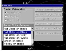
Radar Setup selected from Radar menu (left). Radar Setup menu with Full Color on Black highlighted (right).
